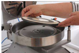
Barely simple exchange of the self-centering discs within seconds
