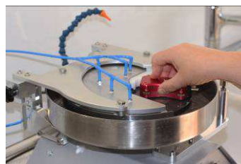
Making thin sections
