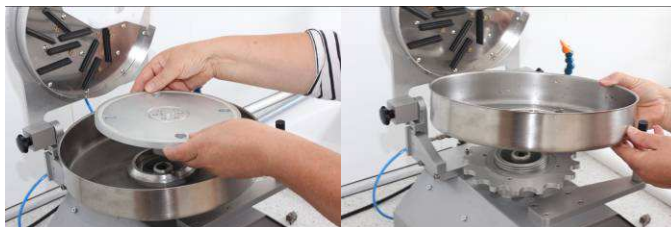
Lightning-fast dismantable without tools
