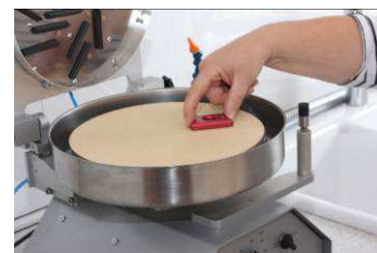
Polishing thin sections
